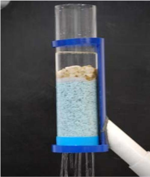
Water has been flowing into the 3" tube for 30 days. Water easily flows through the SPI Media.
