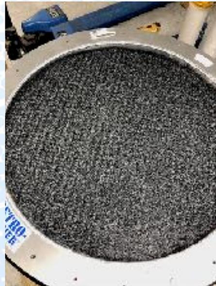
The first layer filtering is flow-free plastic mesh which collects large dirt and prevents it from getting into the next filter. The flow free can be washed and reused.
