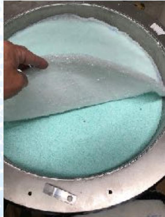
When the Micro Mesh is lifted showing the Petro-Barrier Media. **The purpose of all the dirt filters is to not let dirt into the Media.**
