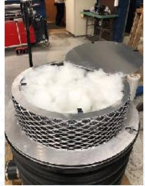
Top-Hat-Filters are attached to the top of the Petro-Barrier Canister with 2 hexed screws and inside the lid is the bags of filtering floss that is then packed into the THF. Flow-free black mesh is attached inside the Top-Hat-Filter, when the floss is installed the lid is closed and is held shut with velcro tape.
