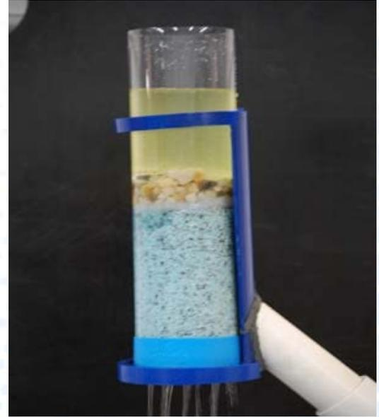
Oil is added to the test demo tube. As the oil is absorbed, the media starts to turn a darker color.
