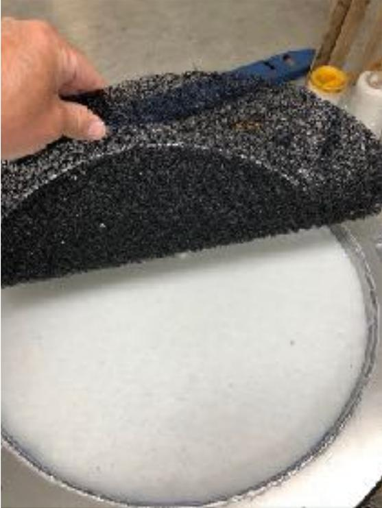
The flow-free mesh is removed from the Petro-Barrier Canister .
