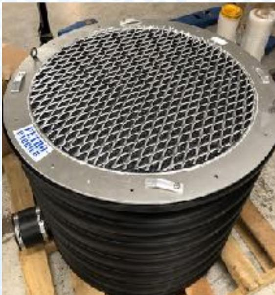
On top of the Petro-Barrier Canister loosen the hex-head screws and slide the 4 - tabs off of the diamond plate grate. Remove the grate.
