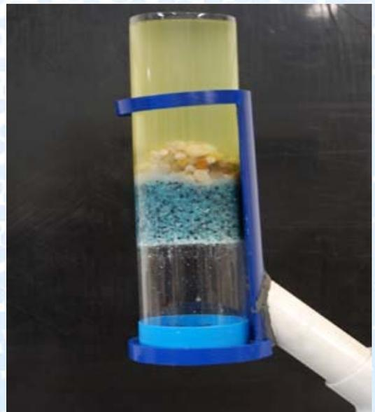
Unused media is removed, leaving only the total seal to illustrate the fact that no water can get through.
